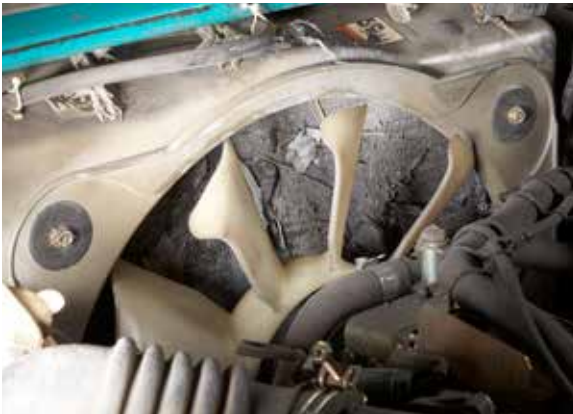
In heavy use applications, some cooling system radiators are compromised by dirt, debris or blowing dust.
